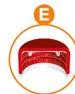
Tamper-evident screw cap with shaped seal
