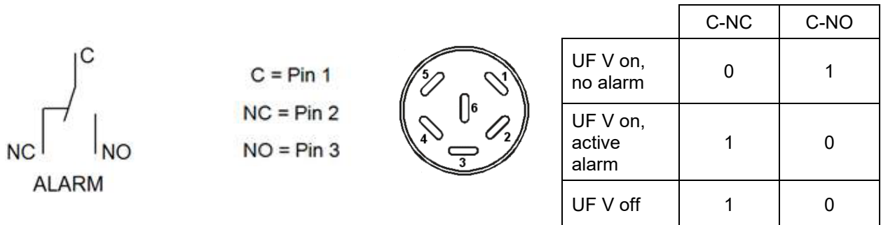
Figure 26: Zero-voltage contacts circuit diagram and pin allocation of DIN socket (9)
