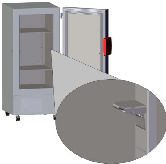
Figure 20: Inserting the shelf holders
