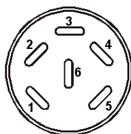
Figure 11: Pin allocation of DIN socket for option analog outputs
